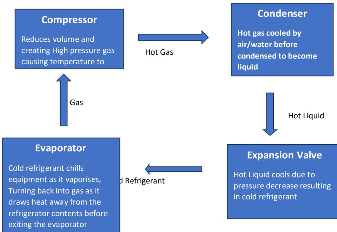
Fig.3 Refrigeration cycle
